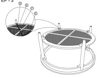
Install the shelf (C) on the legs according to the hole in the leg, Install the JCBC M6 x 40 (F) along with the washer (D) and spring washer (E), (tighten with an allen key (G))
