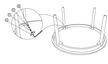
Attach to the 4 legs (B), adjust to the mount on the top(A), then attach the JCBC M6 x 40 (F) with washer (D) and spring washer (E), (tighten with allen key (G ))
