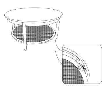
Leveller are provided at the bottom to the balance on uneven surface
